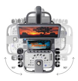
90° right and left ration allows the user the flexibility of choosing the transducer connectors position.
